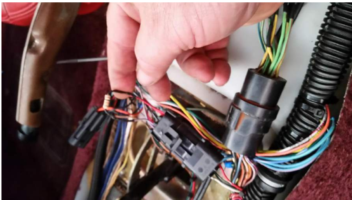
Figure 4 - Wiring in a Pull-Up Resistor in to the VSS Plug
